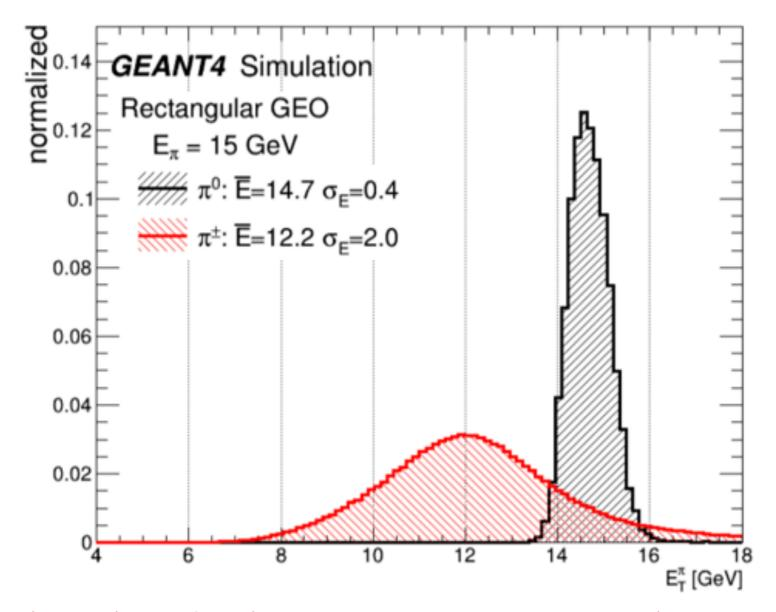
Our GEANT4 simulation takes into account the ATLAS calorimeter granularity, the proper composition of absorber/scintillator material as well as accordion geometry of calorimeter to produce a realistic energy response.
